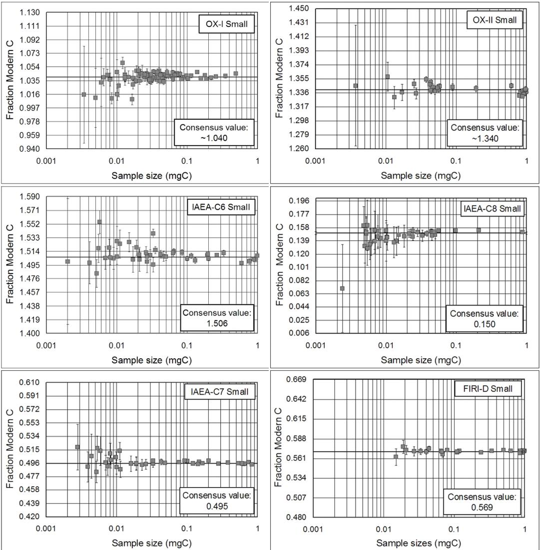
Figure 8 Fraction modern C results for the OX-I, OX-II, IAEA-C6, -C7, -C8, and FIRI-D samples between 0.002 and ~1 mg C from multiple AMS <sup>14</sup>C measurements performed between July 2005 to May 2006 on small and ultra-small sample wheels. Results were normalized and blank corrections applied as for Figure 7.
